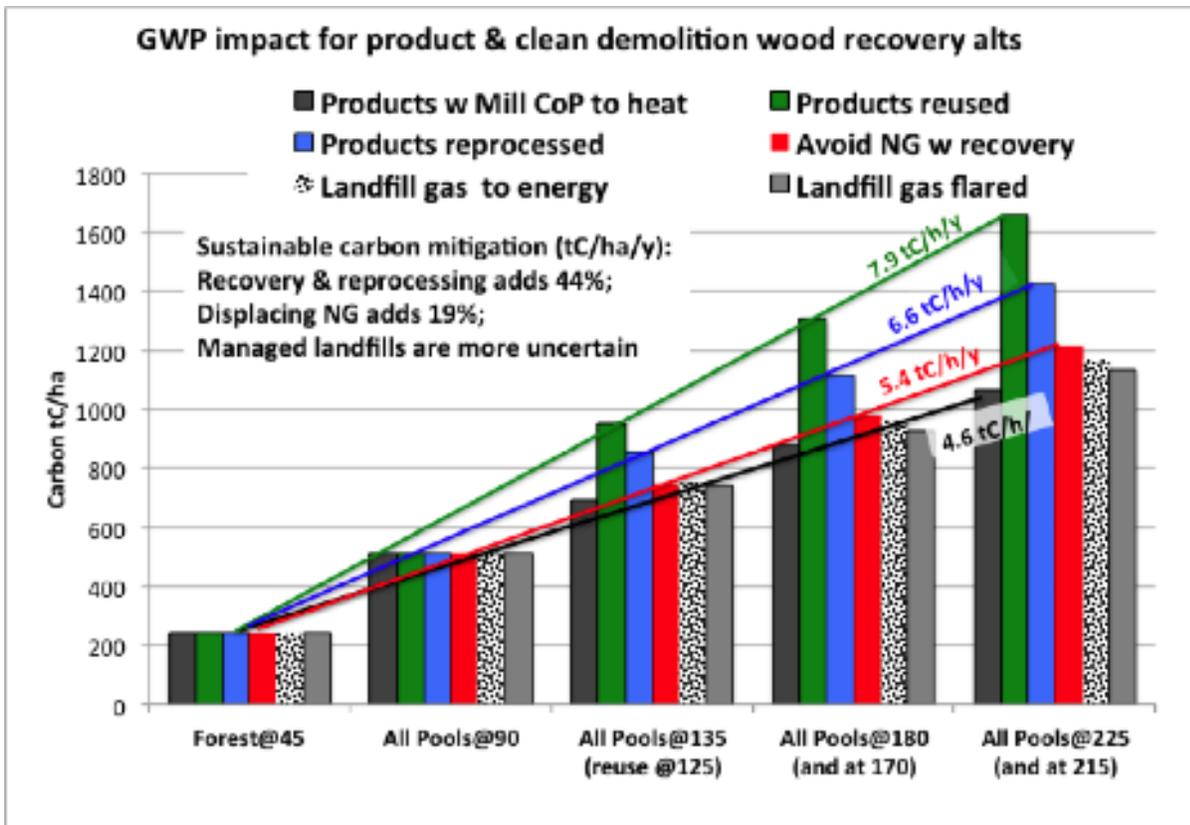
Figure 10. Assessments of sustained carbon mitigation for alternative uses of recovered wood from a PNW forest stand
