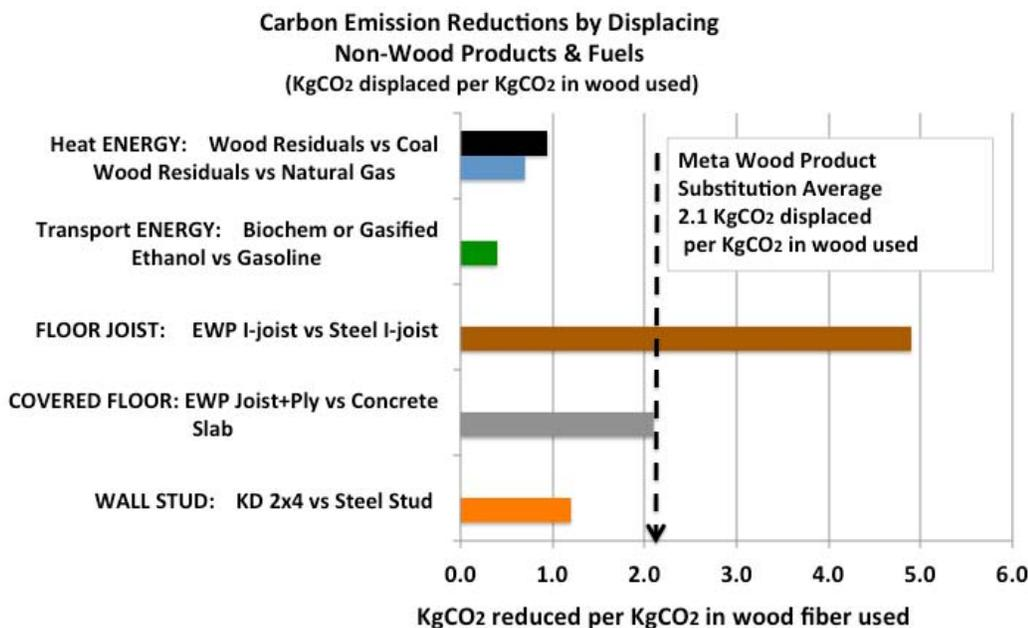
*The substitution of wood for fossil fuel displacing fossil emissions is almost universally accepted, whereas the substitution of wood products for non-wood products is often ignored thereby leaving out the most important aspect of using wood to reduce carbon emissions.*
