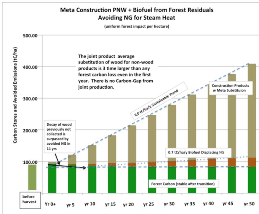
**Figure 8. Total sustainable carbon trend increase from jointly produced wood products and heat from woody biofuel**
