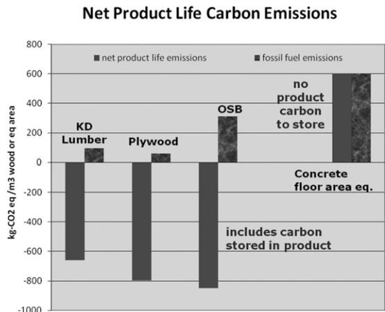
Figure 3. Net carbon emissions, including stored carbon, of a wood floor compared with a concrete floor of the same area. Based on stored product carbon CO<sub>2</sub> equivalent calculated at 1.83 times the dry wood mass.
