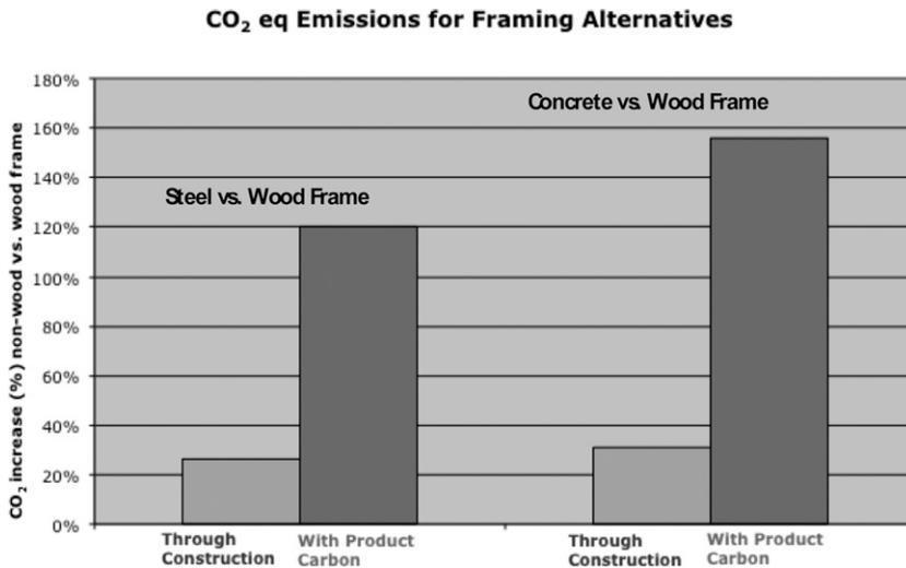
Figure 4. Global Warming Potential carbon equivalent emissions through residential construction for steel and concrete frame vs wood frame ignoring and including the carbon stored in wood products. Based on stored product carbon CO<sub>2</sub> equivalent calculated at 1.83 times the dry wood mass.
