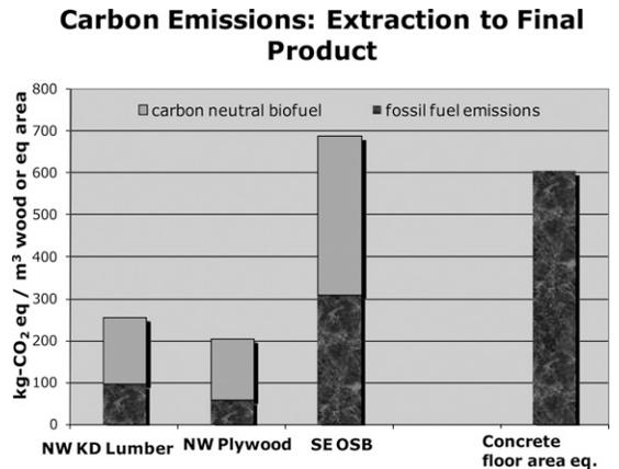
Figure 2. Carbon emissions (as CO<sub>2</sub> equivalents) of a wood floor, from in-ground resources through product manufacturing, compared with a concrete floor of the same area. From Puettmann and Wilson (2005) and Lippke and Edmonds (2006) based on ATHENA EIE analysis of different flooring materials.
