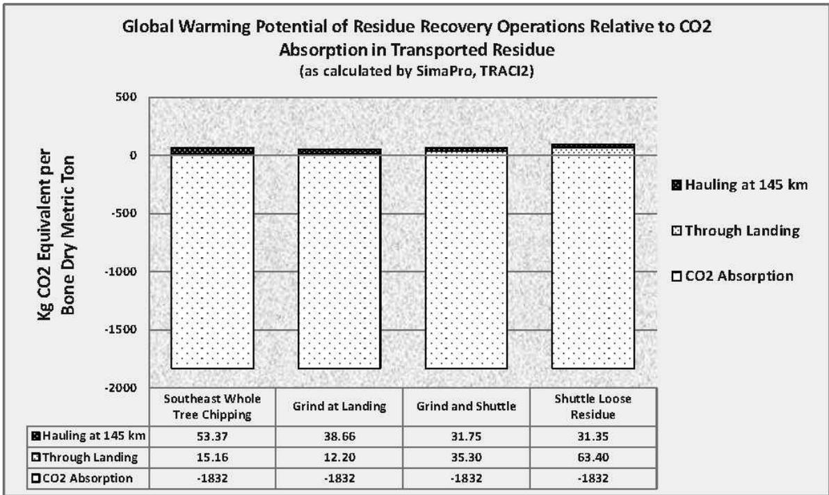
Figure 5.—Net global warming potential of residue recovery operations relative to CO<sub>2</sub> adsorption in the transported material.
