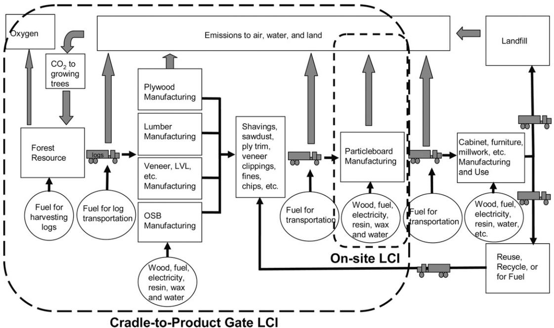
Figure 1. The life cycle of particleboard and its cradle-to-product gate life-cycle inventory system boundary.
