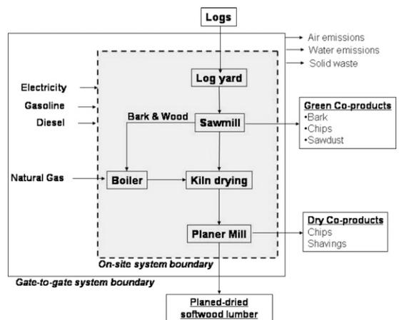
Figure 3. Gate-to-gate system boundary including unit processes used to model Inland Northwest softwood lumber production.
