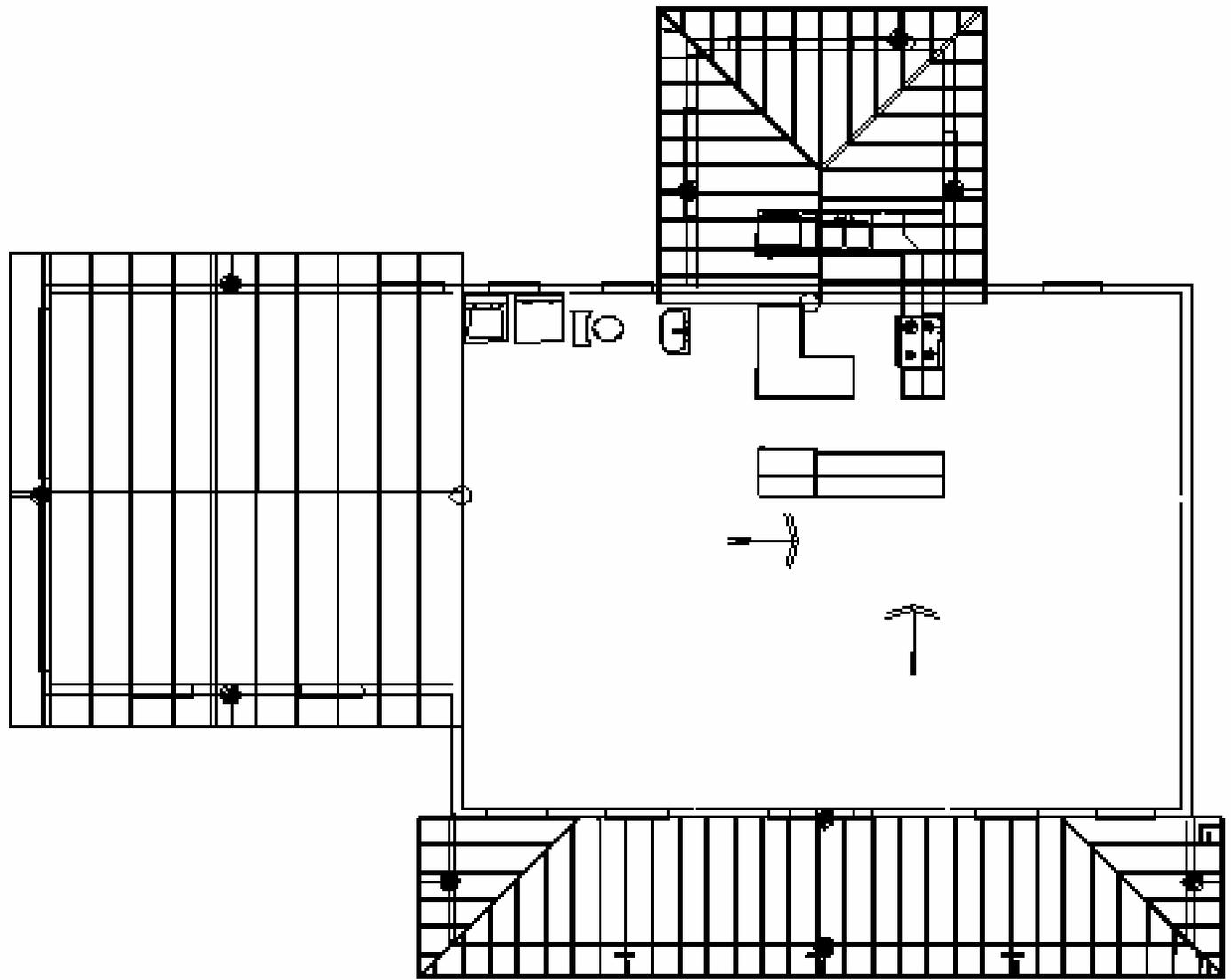
Figure B 8. Minneapolis house - main floor plan with roof and floor framing.
