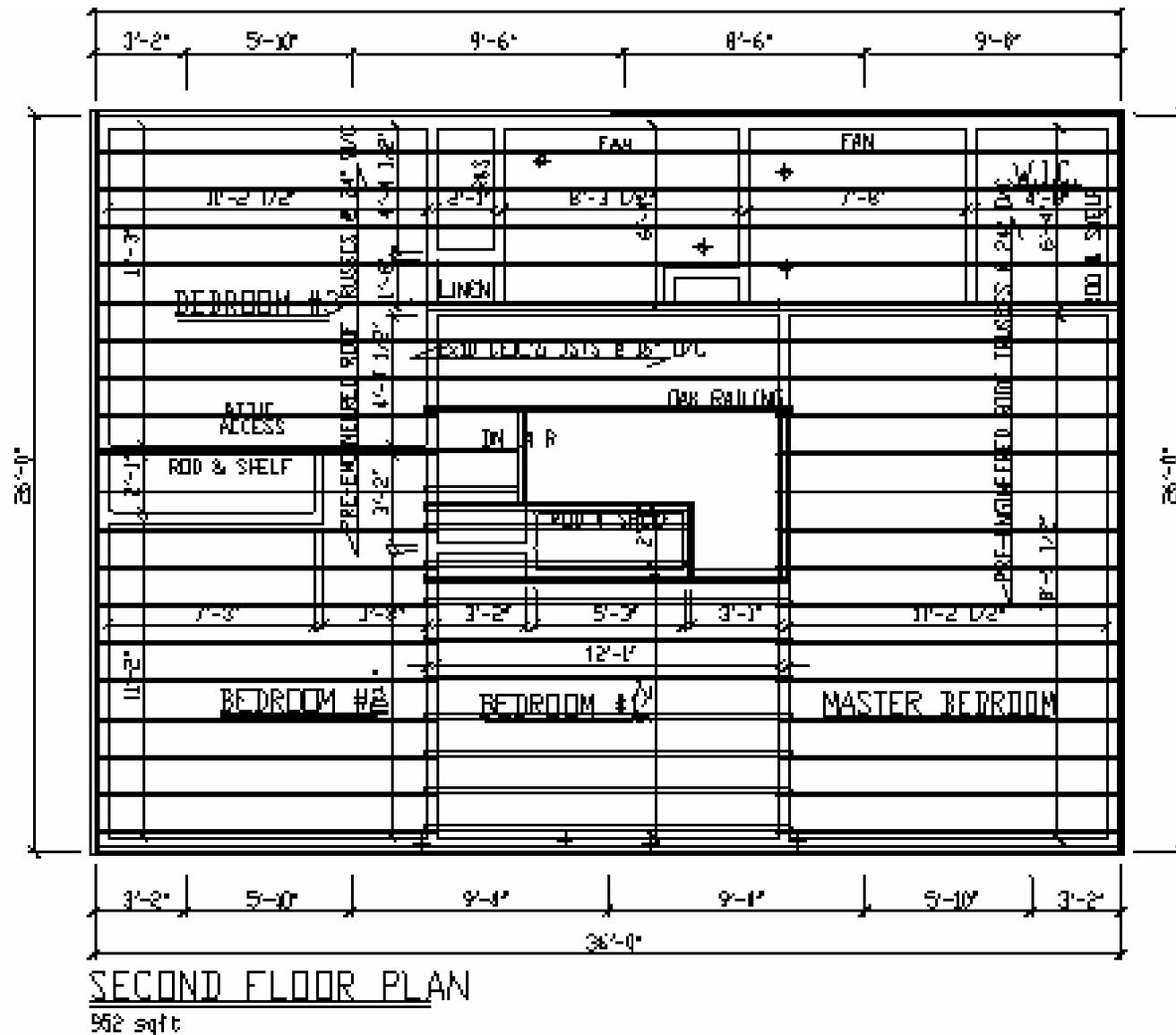
Figure B 10. Minneapolis house - 2nd floor joist framing.
