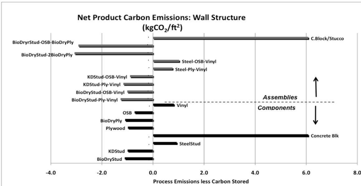
Figure 5.2 Process Emissions less Carbon Stored for Wall Components and Assemblies
