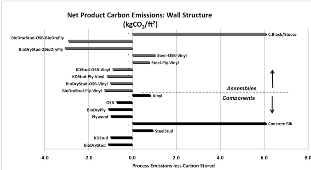
**Figure ES2. Process Emissions less Carbon Stored for Wall Components and Assemblies**
