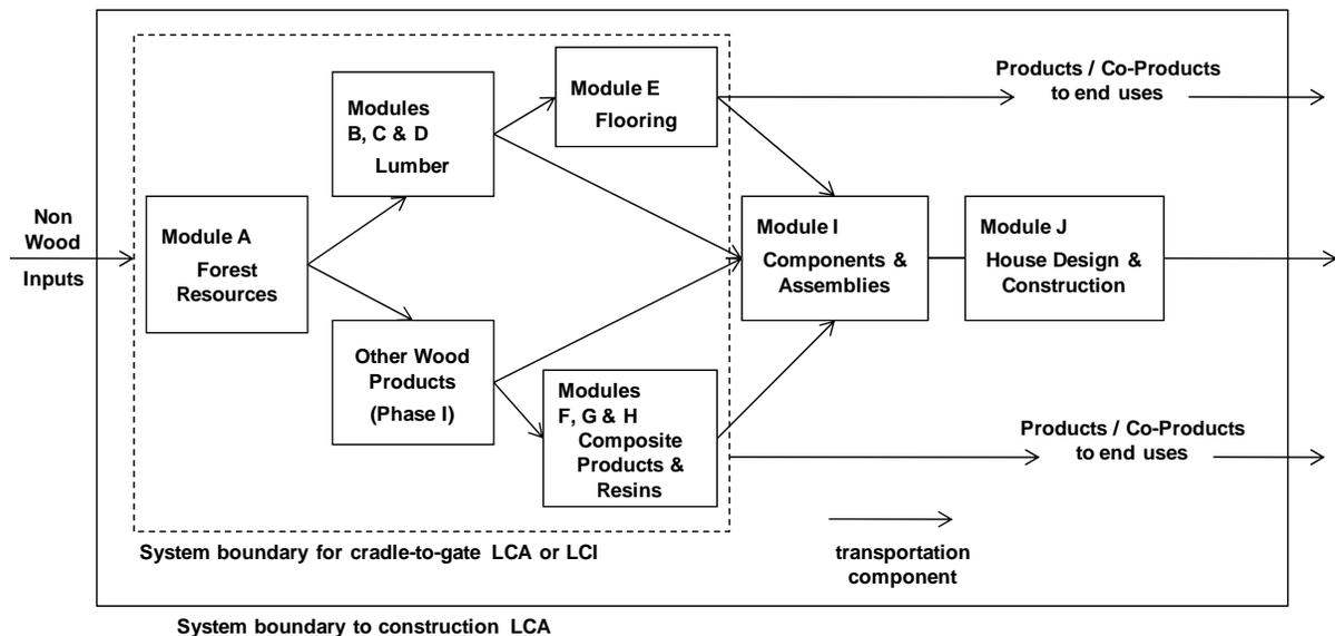
**Figure 3.1 System boundaries used to determine various LCI and LCA values based on LCI data in each report Module**
