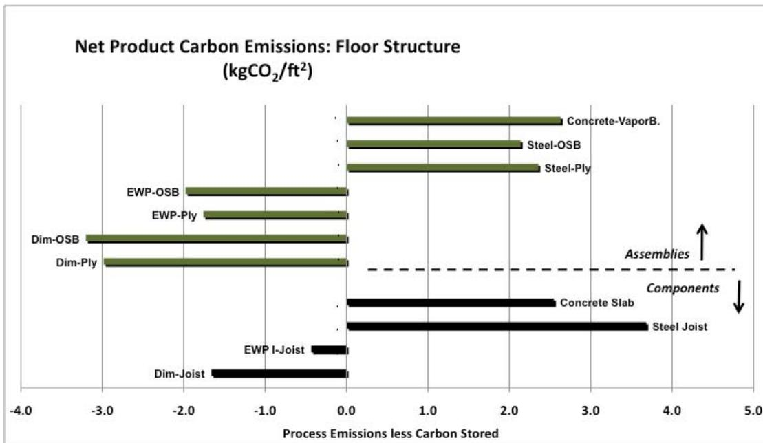
Figure 5.1 Process Emissions less Carbon Stored in Floor Structure Components and Assemblies (source: Appendix Module I)
