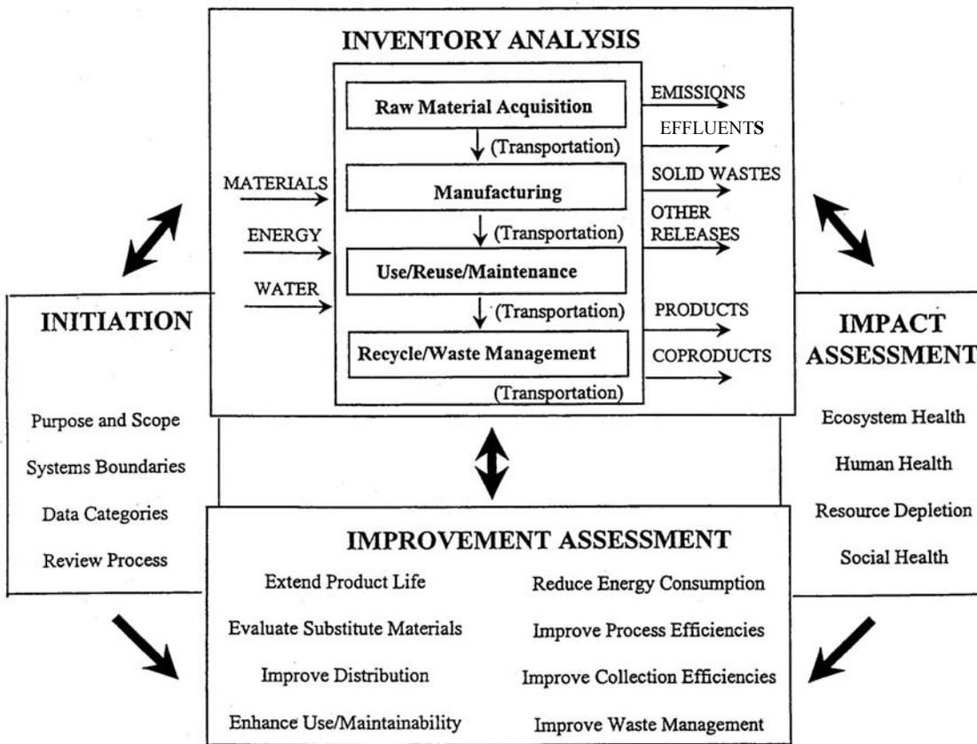
**Figure 2.2 Main Components of an LCA Study**
