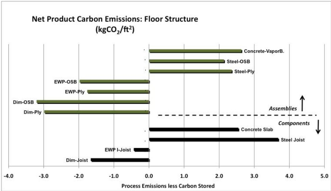
**Figure ES1. Process Emissions less Carbon Stored in Floor Structure Components and Assemblies**
