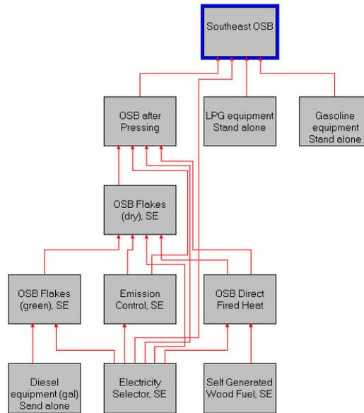
**Figure A2.2. Process tree for only on-site impacts for Southeast OSB manufacturing.**
