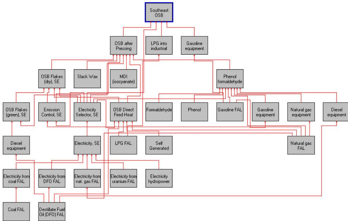
**Figure A2.1. Process tree for both on-site and off-site impacts for Southeast OSB manufacturing. On-site impacts are depicted by the following six processes: Southeast OSB, OSB after Pressing, OSB Flakes (dry), OSB Flakes (green), Emission Control, and OSB Direct Fired Heat processes.**
