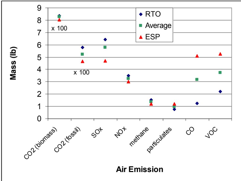
**Figure 5.8.** Off-site and on-site air emissions generated in the production of 1 MSF OSB for RTO, Average, and ESP emission control technologies. CO<sub>2</sub> weight is obtained by multiplying the shown mass by 100.
