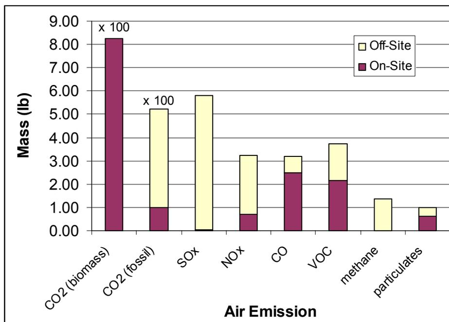
**Figure 5.5. Off-site and on-site air emissions generated in the production of 1 MSF OSB. CO<sub>2</sub> weight is obtained by multiplying the shown mass by 100.**
