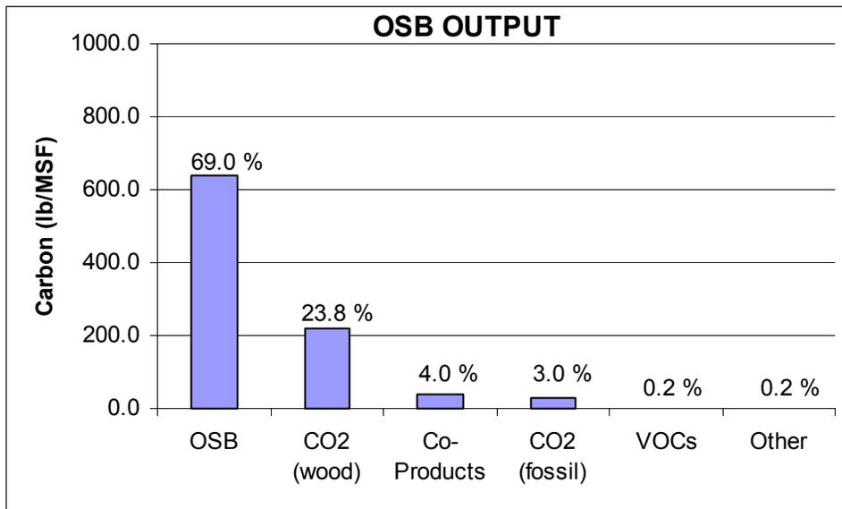
**Figure 5.4. Carbon output destinations for 1 MSF OSB.**
