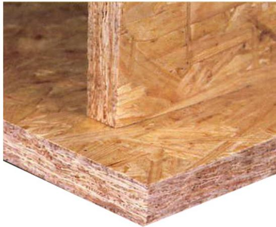
**Figure 1 Oriented strandboard (OSB) panels.**
