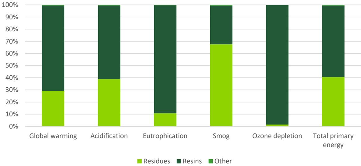
**Figure 6 Cradle-to-gate MDF LCIA Results for A1-Resource extraction (other) and residue and resin production, no allocation, percentage basis, North America.**
