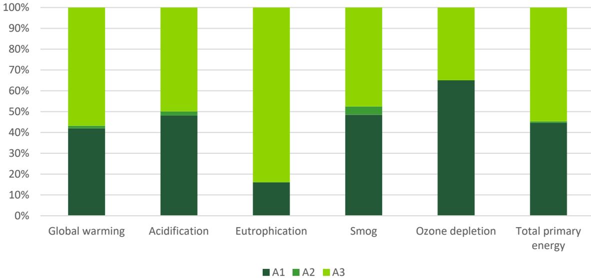
**Figure 5 Cradle-to-gate MDF LCIA Results for A1-Resource extraction and residue and resin production, A2-Transportation, and A3-MDF Production, no allocation, percent basis, North America.**
