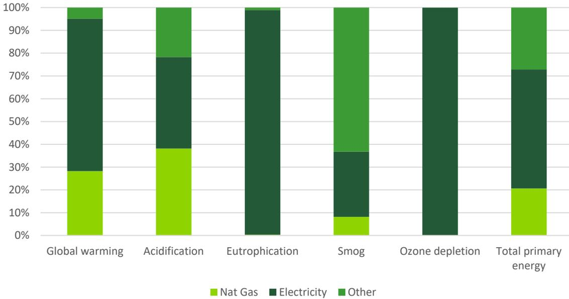
**Figure 7 Gate-to-gate MDF LCIA Results for A3-MDF production, no allocation, percent basis (North America).**
